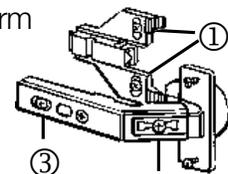
For height adjustments: Loosen screws 2 on hinge plate, adjust door up or down and tighten screws.
