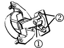
*Easy Reach Hinges* - For side adjustments: Locate the concealed Phillips head screw 2. Turn to desired adjustment. For height adjustments: Loosen screws 1 on hinge plate, adjust door up or down and tighten screws.
