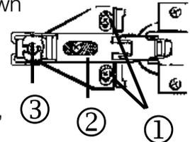
For forward or backward movement, adjust Phillips head screw 3 at the end of hinge arm.
