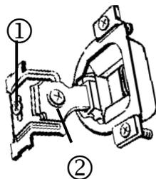
For height adjustments: As shown here, simply loosen the screws 1 and 2 attaching the hinges to the frame and move the door up or down to the desired position.
